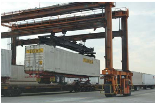
Trailers Lifted Onto Flat Wagon at BNSF Willow Springs Multimodal Hub
