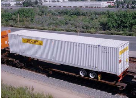
Container Coupled with Chassis Moving as Trailers to Reduce Transit Time
