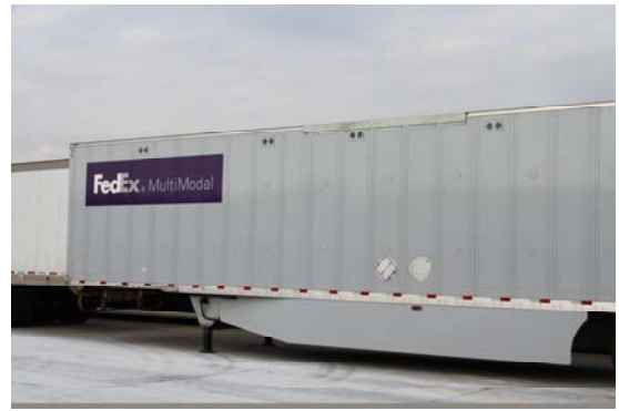
FedEx Trailer with Side Skirt to Reduce Drag
