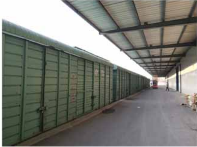
Rail sidings along warehouses in a logistics park in Tashkent. Often warehouses are designed with one side for rail and the opposite side for trucks.
