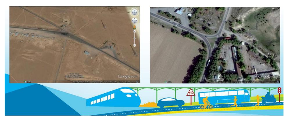
Y junctions should be eliminated by converting to T junctions.
