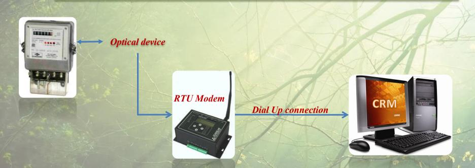
Reading data manually with an optical device.
