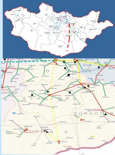
Project name : **UB-Oyu tolgoi power line** Project venue : Power line Ulaanbaatar - Oyu tolgoi gold and copper mine, 560km Production scale : 220 kV, 100MW Total investment : 150 million US\$ Market orientation and market analyses : Power supply for Oyu tolgoi gold copper mine from the CES
