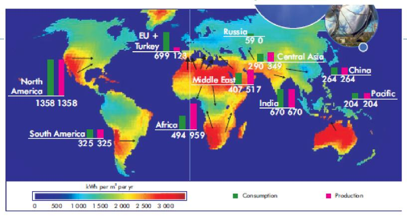
Repartition of the direct normal irradiance (DNI) in kWh/m<sup>2</sup>/y, and of the production and consumption of CSP electricity (in TWh) by world region in 2050 as foreceen in this roadmap. Arrows represent transfers of CSP electricity from sunniest regions or countries to large electricity demand centres.
