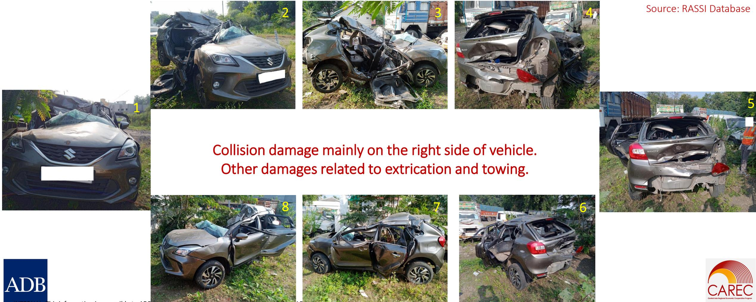
Collision damage mainly on the right side of vehicle.
