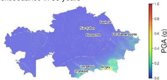
Figure 18: Seismic hazard map for peak ground acceleration (PGA) with a 10% probability of exceedance in 50 years
