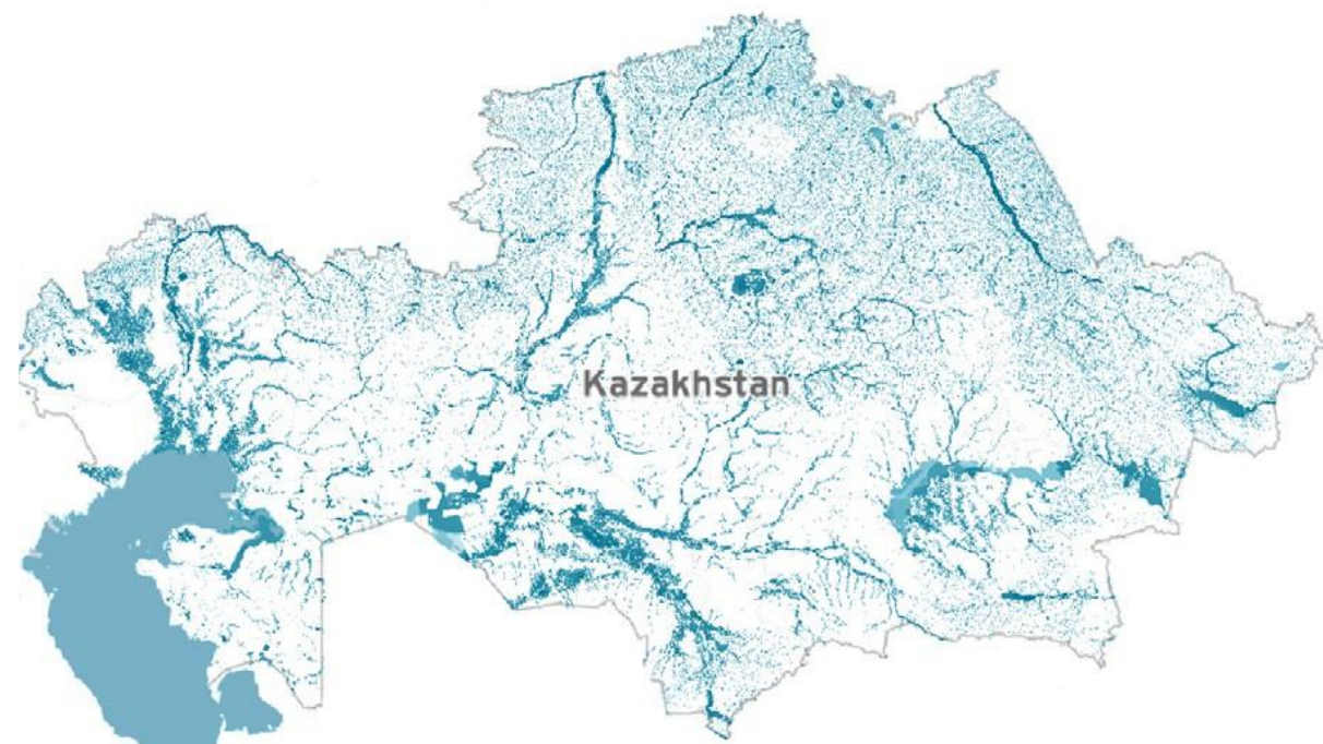
Figure 21: Map of river (fluvial) flooding (areas in blue) at the 200-year return period level
