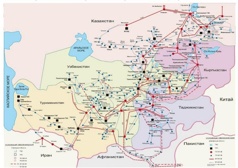
• At present the CA UES consists of the energy systems of South Kazakhstan, Kyrgyzstan and Uzbekistan, that work in parallel with the Unified energy system of Russia and the CIS through Kazakhstan's energy system.
