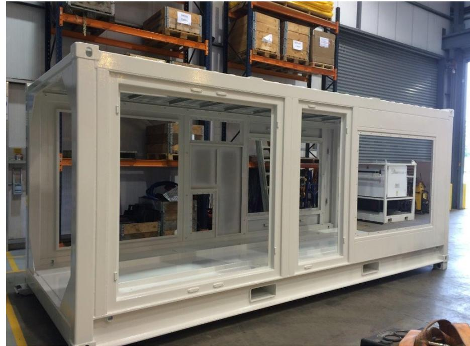
Container modules are custom built – certified for shipping with equipment installed
