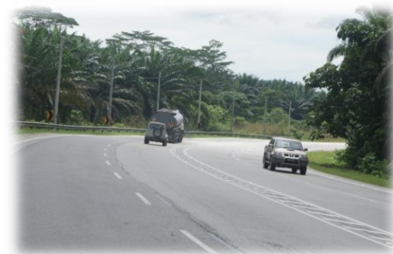
iRAP proposed countermeasure: Central hatching on rural primary roads
