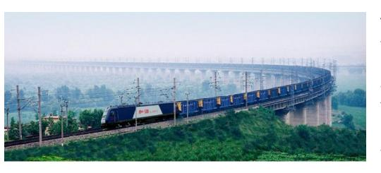
The Datong-Qinhuangdao railway is the first electrified double-track coal line in China. With a traffic volume of 445 million tons in 2013, it became the heavy haul railway with the largest annual traffic volume in the world. In April 2014, the trial operation of 30,000t heavy haul train was carried out on the Datong-Qinhuangdao railway.
