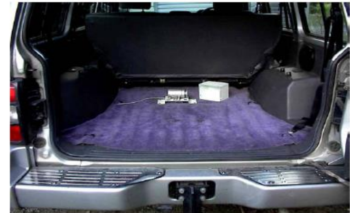
ROMDAS BI Installed in Vehicle With Protective Cover Off
