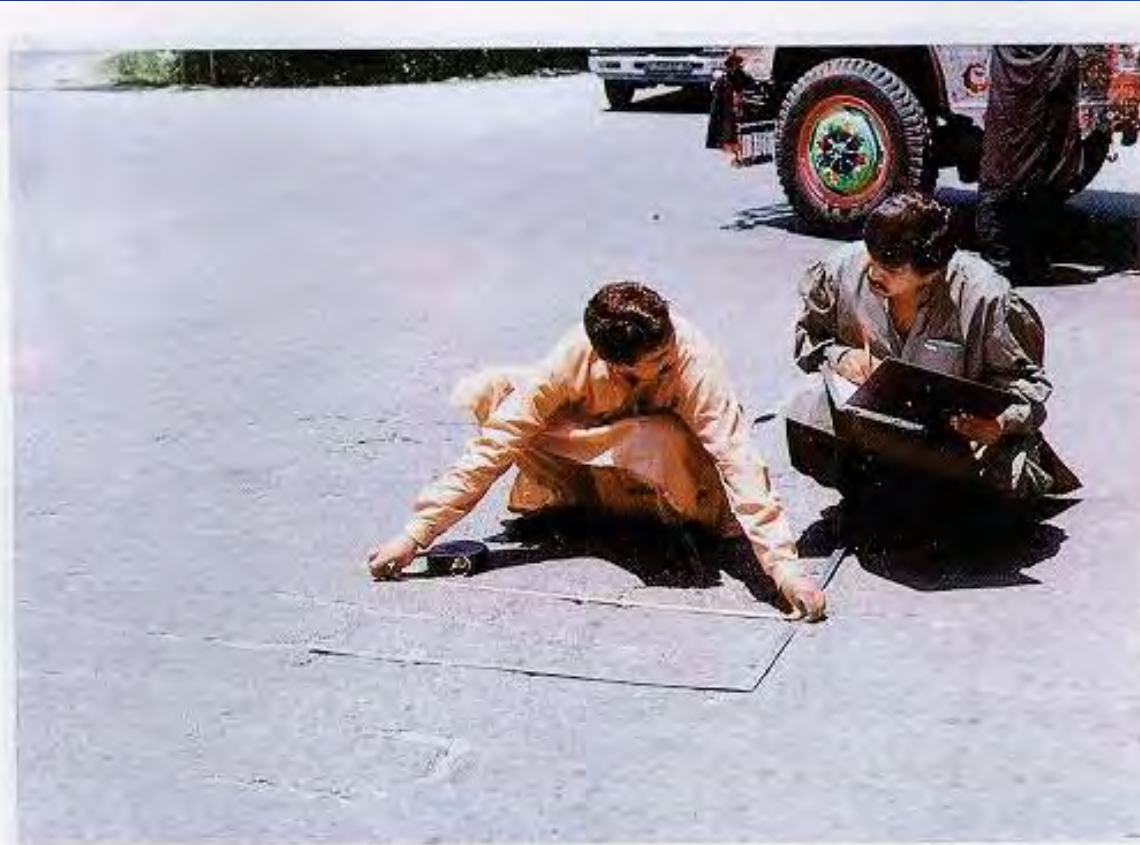
Figure 4. PAVEMENT CONDITION SURVEY (CRACK MEASUREMENT)
