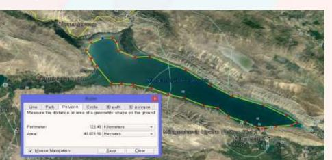
The Mingachevir HPP is the largest in the country, with an installed capacity of 420 MW. The reservoir is built in 1953, is 75m at maximum depth and the capacity of 15.73 km³. Average depth is 26m and the shore length is 247 km. The overall area of the reservoir is 605 km². (Theoretical capacity: 40,000 hectares = **40 GW**)
