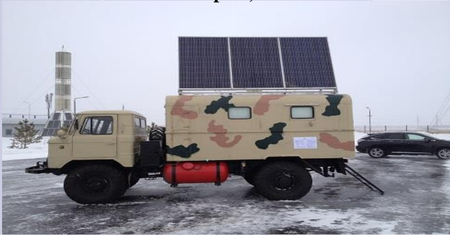
Mobile solar installation for hunters, fishermen, beekeepers, 0.8 kW
