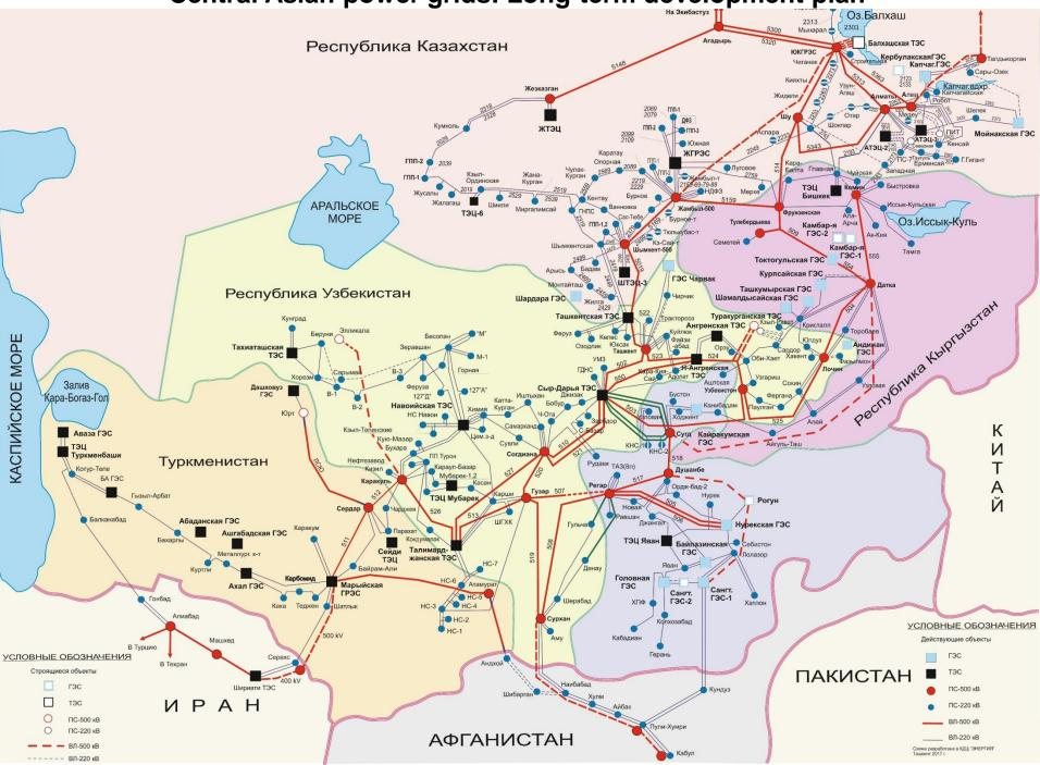
•At present, the power grids of the Southern part of Kazakhstan, Kyrgyzstan and Uzbekistan operate within the Central Asian Interconnected Power Grid (CA IPG). Through the power grid of Kazakhstan, they operate in parallel with the Unified Power Grids of Russia and the CIS.
