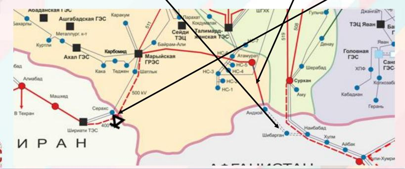
• For example, such a link through a 500/400 kV back-to-back station exists between power grids of Georgia and Armenia (Georgia works in parallel with Russia, while Armenia works in parallel with Iran and Turkey)
