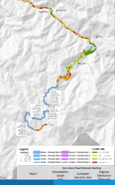
The selection of possible road project candidates starts with visualization (GIS- map) of the obtained results from HDM 4 program analysis. The possible of road project candidates are presented on the map as homogenous road sections with information on; condition, traffic data, estimated costs for maintenance/ rehabilitation, expected benefits in relation to the costs, and population density.
