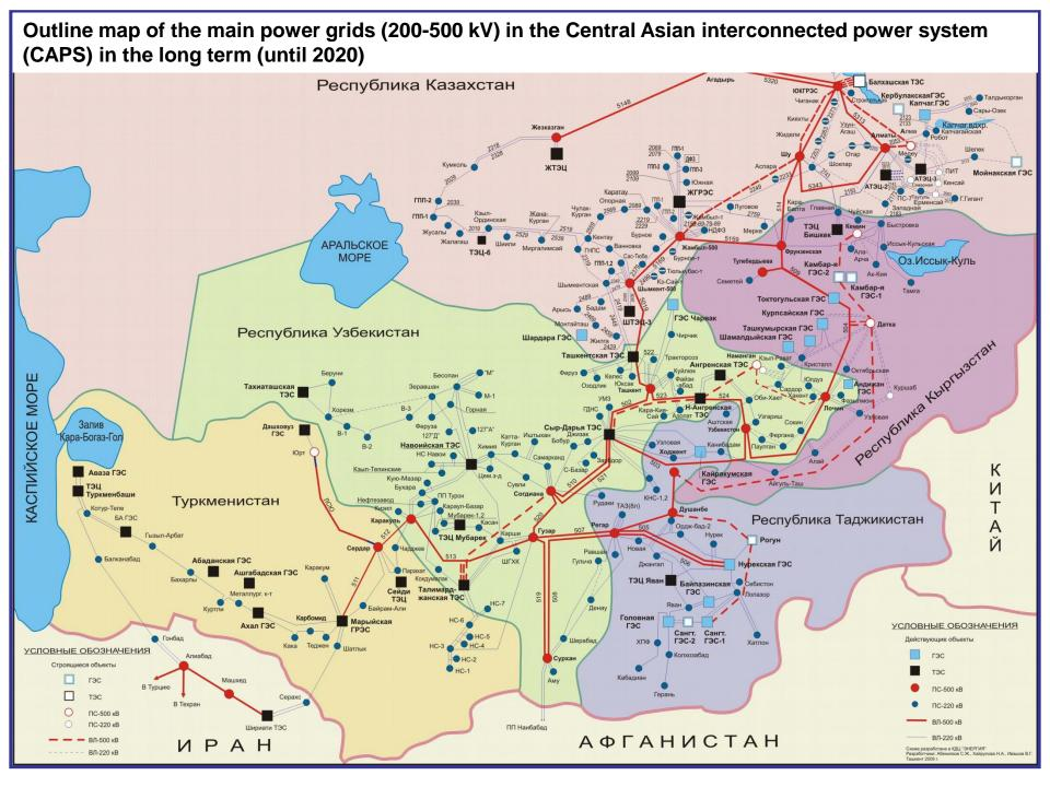
• At present, power systems of Uzbekistan, Kyrgyzstan and the Southern Kazakhstan operate in parallel in CAPS. CAPS is synchronized with the Unified Energy System (UES) of the CIS through the UES of Kazakhstan.
